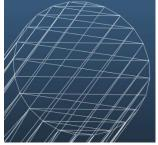
• We can fix the problem by **projecting** all triangles onto the facet's plane. Select the triangles and open the Mirror / Project command:
